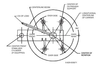
Bold lines determine the limiting position of any load for operation within working areas indicated.
