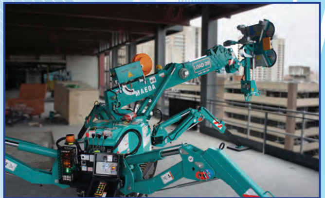
Oktopus Remote Control Glass Lifter Optional - All MC Models 1,322 lb. (600kg) Max. Capacity
