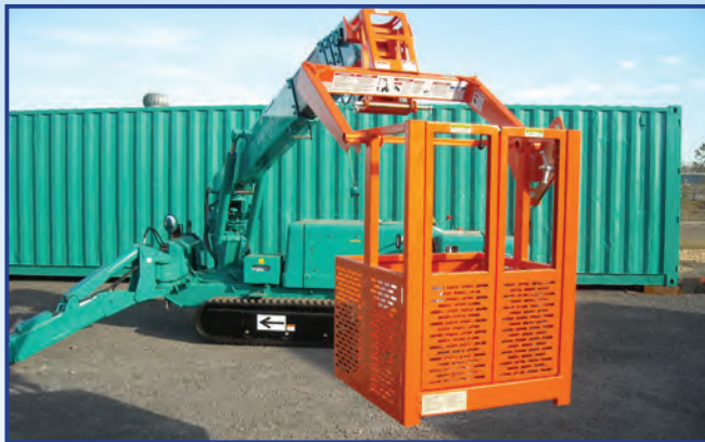
Man Basket Optional - All MC Models 300 lb. (136kg) Payload Capacity
