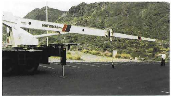
The sequence of photos above shows how the National 1200 29-52 foot jib folds out into a working position.
